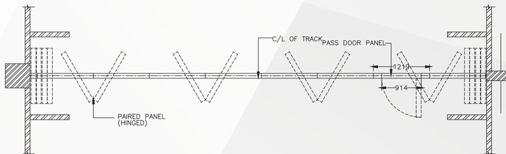
Select for wall-to-wall space division. Panels are hinged in pairs allowing fast setup. They may be stacked at either or both ends of the track or in a "pocket". One or more pair of panels may also be placed anywhere along the track for use as sight dividers.
